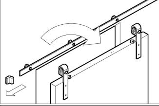
STEP 4: Install the Soft Close in correct orientation. (Illustrated from the rear, soft close can easily be unscrewed and reversed to get correct orientation).
