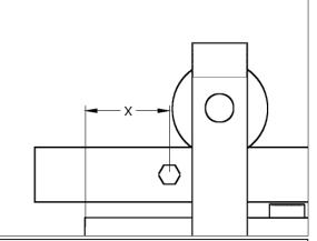
**STEP 3**: Drill pilot holes for the trigger in the position below (X is taken from **STEP 1**).
