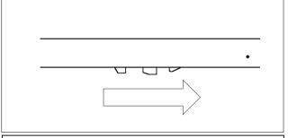
STEP 11: Check the engagement of the trigger with the Soft Close jaws. Adjust the trigger height as necessary.
