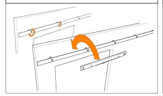
**STEP 6**: The Soft Close sits behind the track. Tighten the two fixings.
