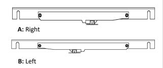
STEP 5: Loosen end two fixings. Slot Soft Close onto standoffs.
