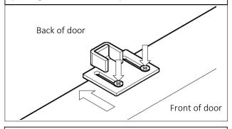
STEP 8: Hang the door back on the track, ensuring the floor guide is engaged.
