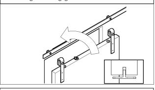
STEP 9: Adjust the trigger into the final position and tighten the screws.
