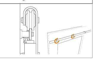
STEP 7: Loosely install the trigger on top of the door pushing it as far forward as possible.
