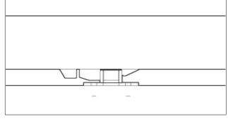
**STEP 12:** Check the anti-jump cams are engaged. Replace the door stop to the ends of the track.
